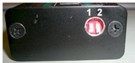
Figure 4 DIP switches and advance curve selection.
