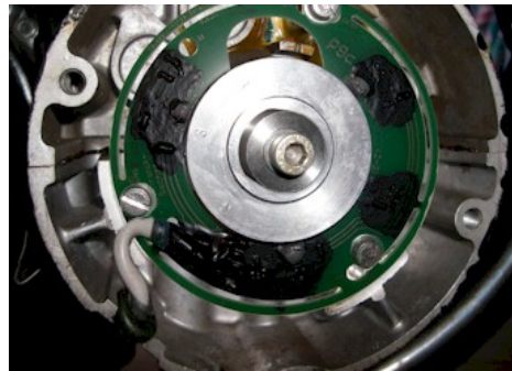
Figure 2 Installed pickup + driver sleeve + magnet disk.
