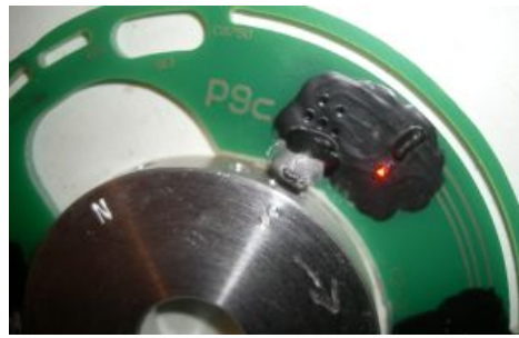
Figure 8 The LED goes on when the S-magnet passes the sensor.
