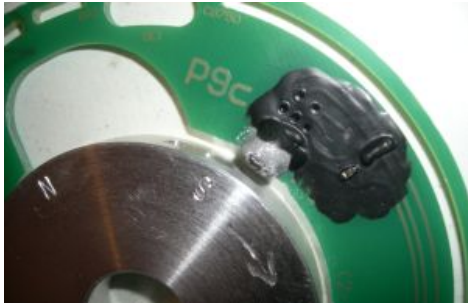
Figure 8 Position the magnet disk, so the sensor is just in front of the S-magnet.
