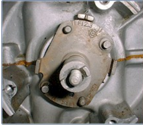
Figure 2.a Using the original sleeve with our magnet disk. This is the recommended method if this kit includes no driver sleeve.
