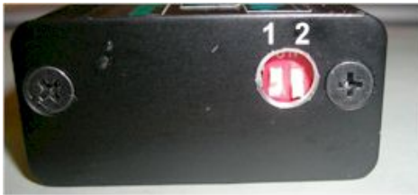
Figure 6 DIP switches and advance curve selection.
