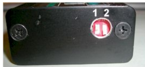
Figure 4 DIP switches and advance curve selection.
