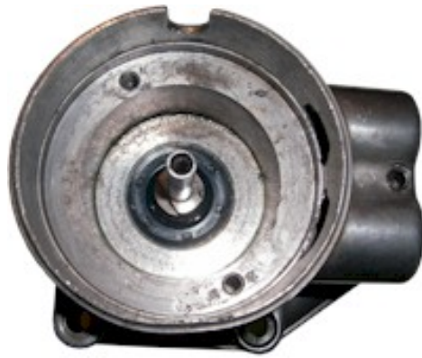
Figure 2 Removal of the old ignition components.
