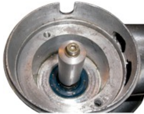
Figure 2 Mounting the driver sleeve on the shaft.
