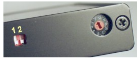
Figure 4 DIP switches and rotary switch.
