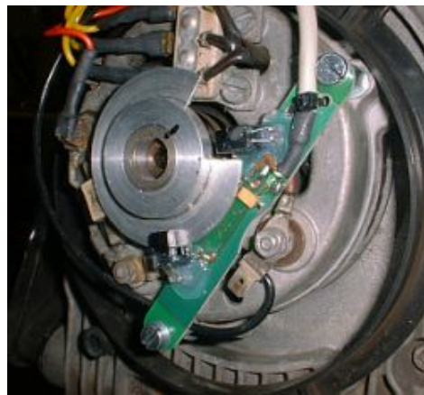
Figure 5.h Installed pickup and sector disk
