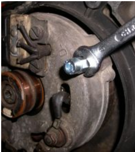
Figure 5 Mounted spacer on the rods
