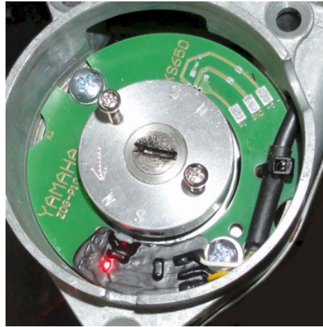
Figure 6 The LED goes on when the S-magnet passes the sensor and off when the N-magnet passes the sensor.
