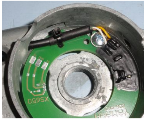
Figure 2 Mounting the pickup.
