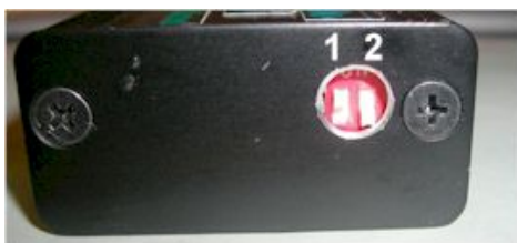
Figure 4 DIP switches and advance curve selection.
