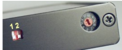
Figure 5 DIP switches and rotary switch.
