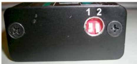
Figure 4 DIP switches and advance curve selection.
