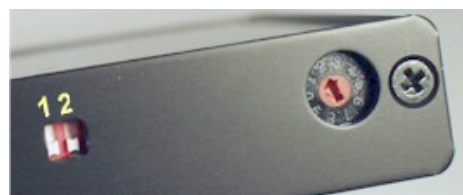
Figure 5 DIP switches and rotary switch.
