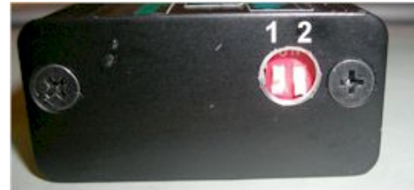
Figure 5 DIP switches and advance curve selection.
