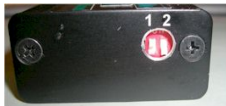
Figure 5 DIP switches and advance curve selection.
