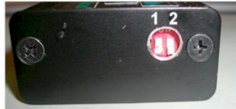
Figure 5 DIP switches and advance curve selection.
