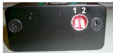
Figure 4 DIP switches and advance curve selection.
