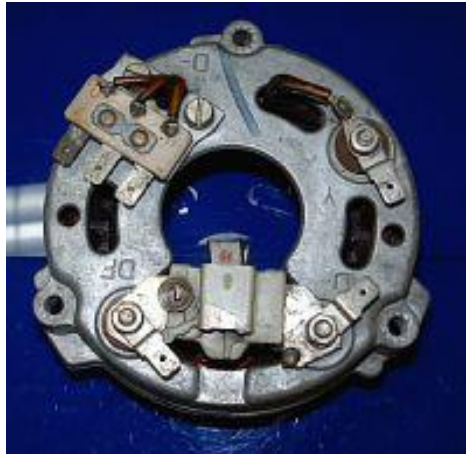
Figure 2 Remove the connector block and Y-connection.
