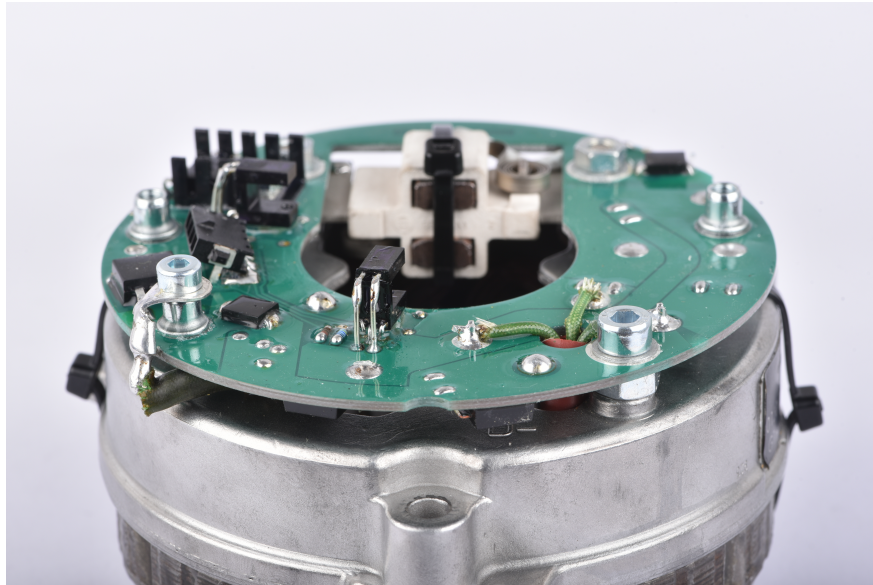
Figure 6 The mounted regulator
