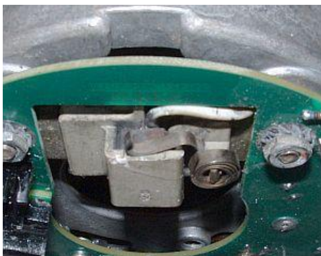
Figure 5 Unclip the brusher spring
