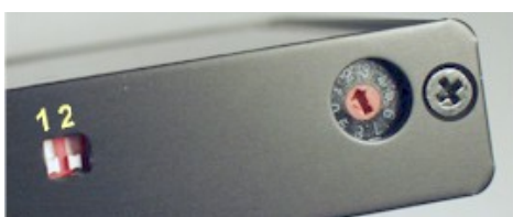
Figure 15 DIP switches and rotary switch.
