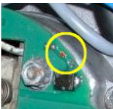
Figure 12 LED for the regulator circuit.
