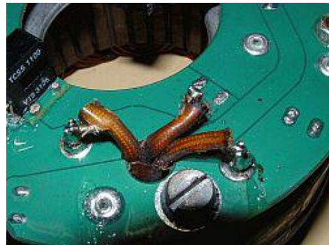
Figure 4 Solder the three wires from the alternator.
