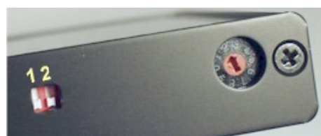
Figure 7 DIP switches and rotary switch.
