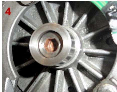
Mounting the drive sleeve hub
