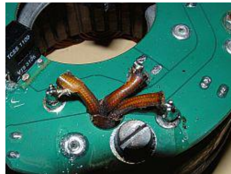
Figure 3 Solder the three wires from the alternator
