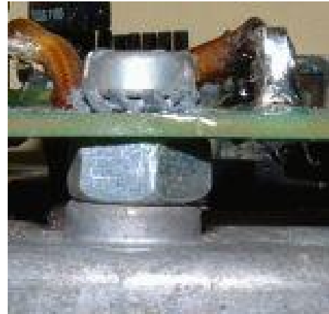
Figure 2 Use the nut as spacer
