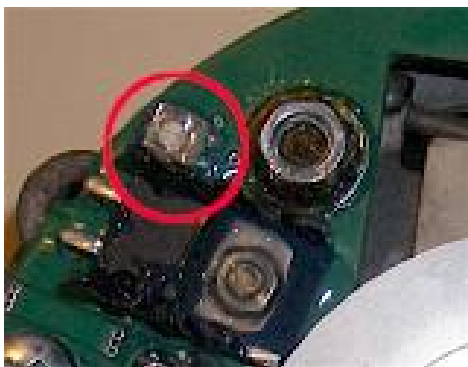
Figure 7 Trimmer to select charging voltage.
