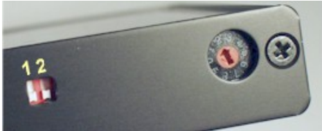
Figure 4 DIP switches and rotary switch.
