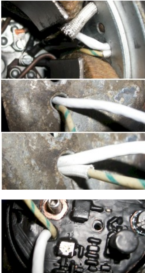
Cable routing through the regulator base plate (in this picture the regulator RegKS is shown)
