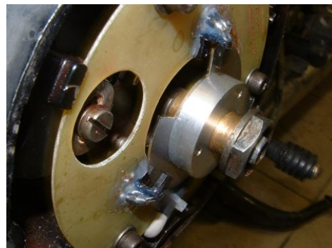
Figure 2.e Alignment of the magnet disk to the sensors (note that the image shows an older version).
