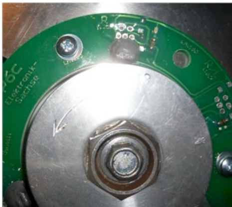
Figure 8 When the N-magnet passes, the LED turns off.
