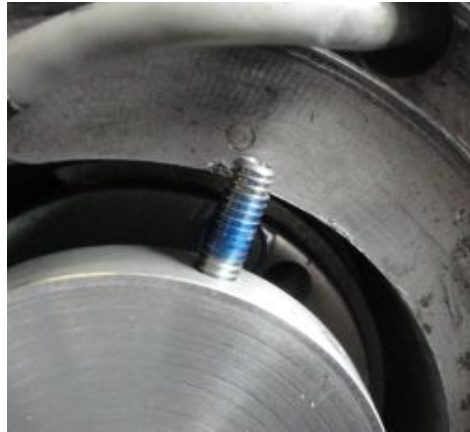
Figure 7 Use medium strength thread lock compound for the set screws.
