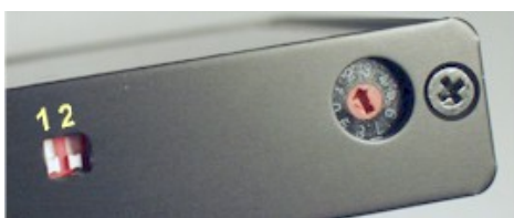
Figure 4 DIP switches and rotary switch.
