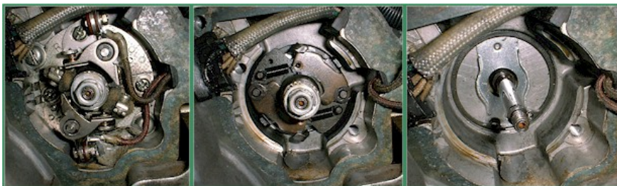
Figure 2 Removing the old parts or the original ignition.
