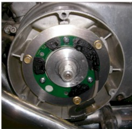
Figure 2 Complete assembly of pickup
