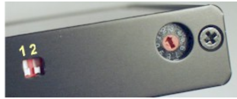
Figure 10 DIP switches and rotary switch.
