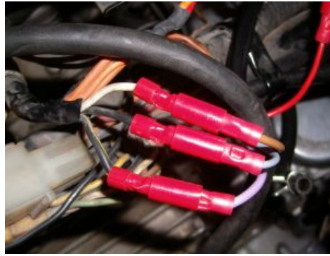
Figure 5 Coil cable connection.
