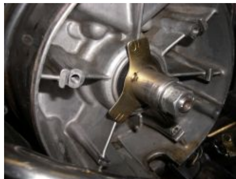
Figure 2 Removal of the old ignition components.
