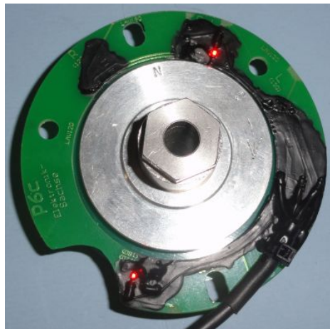
Figure 6 Pickup with driver sleeve and magnet disk.
