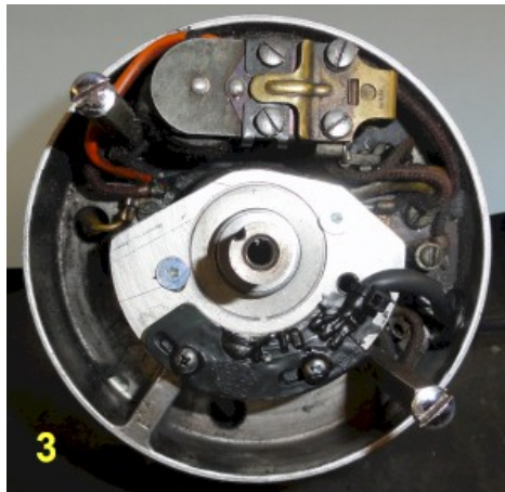
Figure 2 Mount the new pickup.
