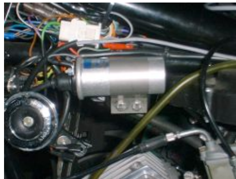
Figure 2 Mounting suggestion with PVL220 ignition coils.
