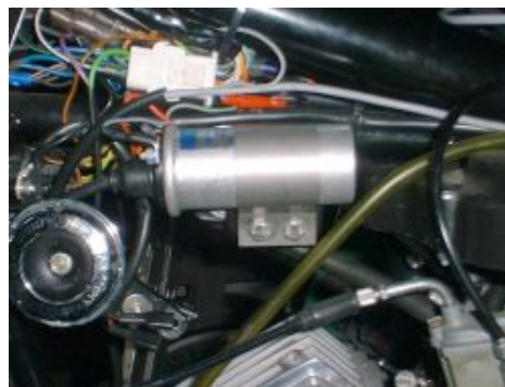
Figure 2 Mounting suggestion with PVL220 ignition coils.
