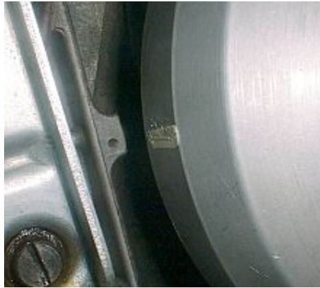
Figure 6 Set the rear piston to TDC.
