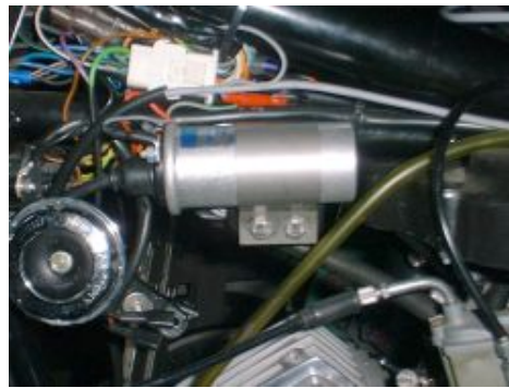
Figure 2.d Mounting suggestion with PVL220 ignition coils.
