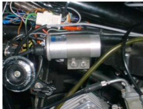
Figure 2 Mounting suggestion with PVL220 ignition coils.
