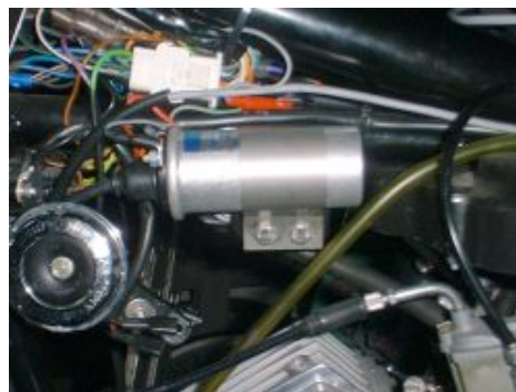
Figure 3 Mounting suggestion with PVL220 coil
