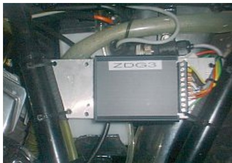
Figure 3 Mounting the ignition box
