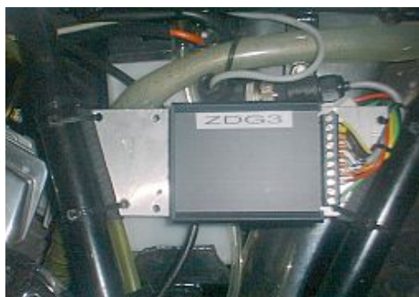
Figure 3 Mounting the ignition box
