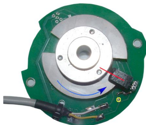
Figure 7 Pickup with magnet disk (figure shows older version).
