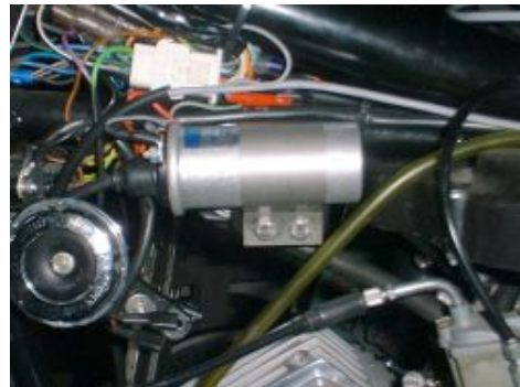
Figure 3 Mounting suggestion with PVL220 coil
