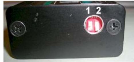
Figure 4 DIP switches and advance curve selection.
