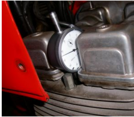
Figure 6 Dial gauge to precisely find TDC.
