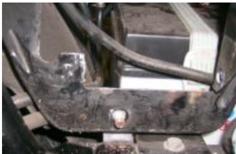
Figure 2.j Mounting suggestion for the ignition box.
