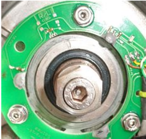
Figure 2.g The pickup is mounted.
