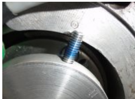
Figure 6 Use medium strength thread lock compound for the set screws.
