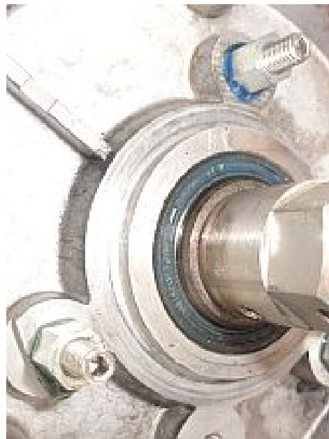
Figure 2 Spacers are put in place.
