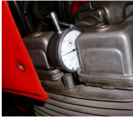
Figure 6 Dial gauge to precisely find TDC.
