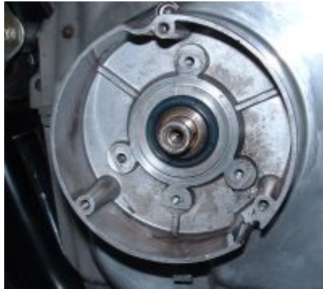
Figure 2 Removal of the old ignition components.
