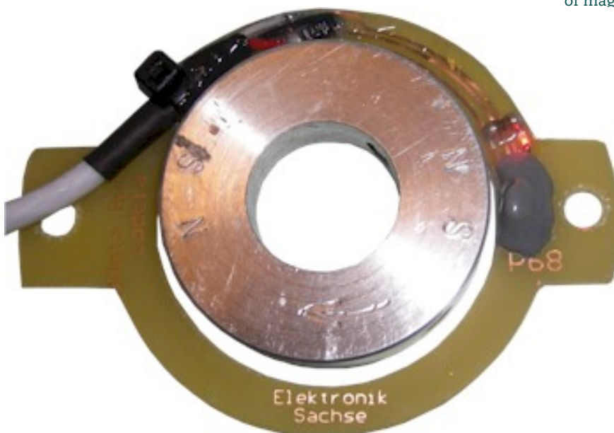
Figure 3 Ensure correct alignment of magnet disk and sensor.
