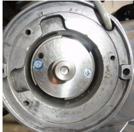
Figure 2.b Mounting the driver sleeve
