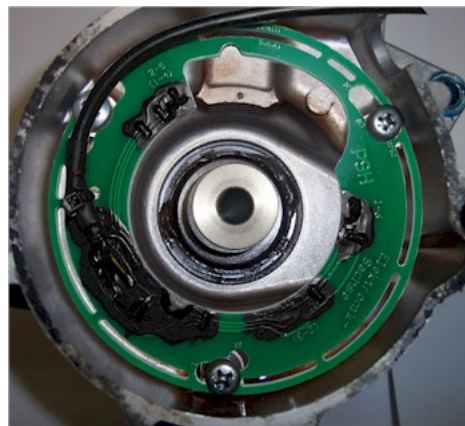
Figure 2 Mounted pickup and driver sleeve. The magnet disk is not mounted, yet.
