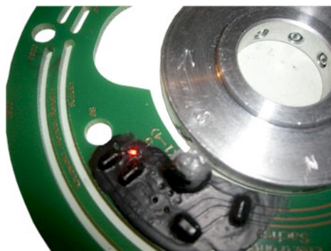
Figure 6 The LED goes on when the S-magnet passes the sensor and off when the N-magnet passes the sensor.
