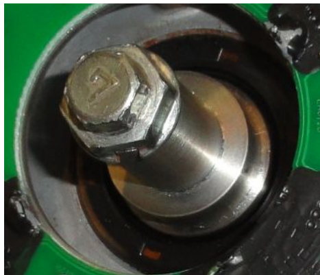
Figure 2 Mounting the driver sleeve.
