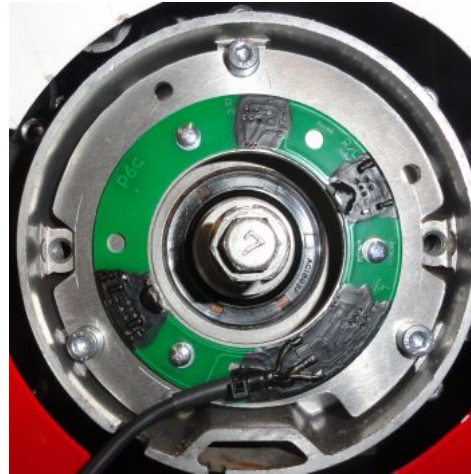
Figure 2.b Mounting the new pickup with the base plate.
