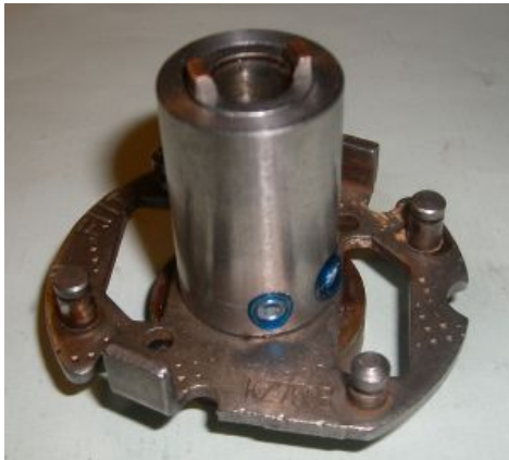
Figure 2 Driver sleeve mounted on the original shaft.
