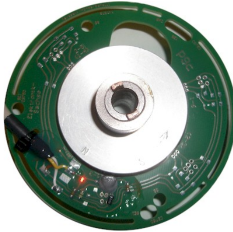
Figure 7 Pickup with driver sleeve and magnet disk.
