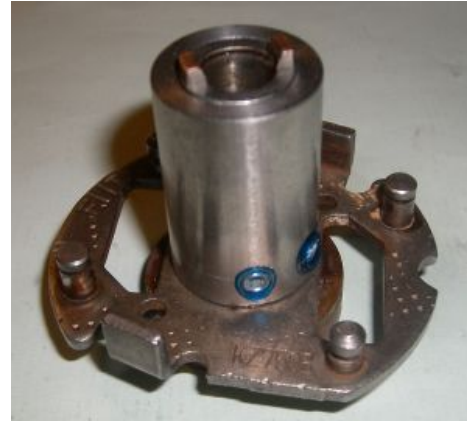
Figure 2 Driver sleeve mounted on the original shaft.
