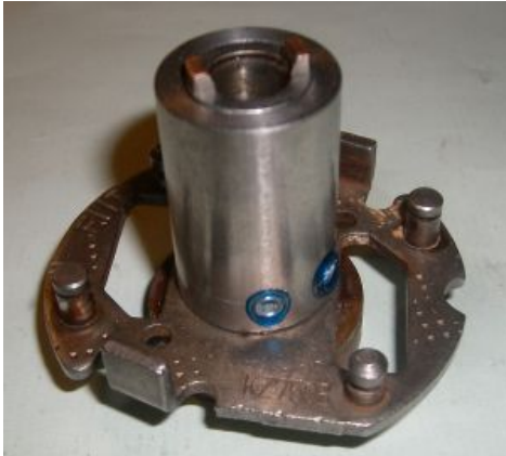
Figure 2 Driver sleeve mounted on the original shaft.
