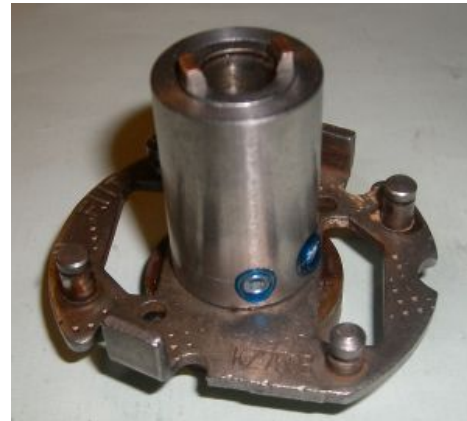
Figure 2 Driver sleeve mounted on the original shaft.
