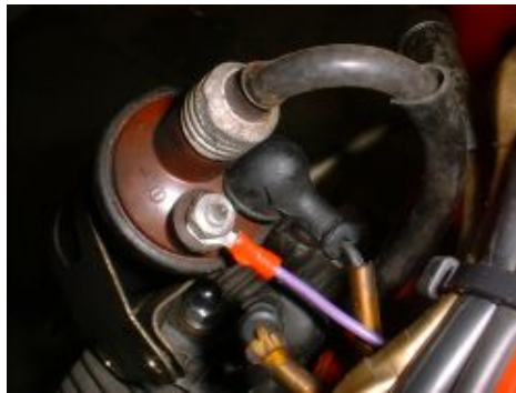
Figure 3.b Mounting suggestion of the left ignition coil.
