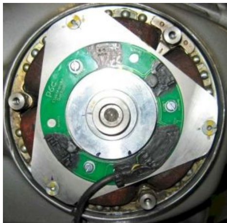
Figure 2 Mounting the pickup (image shows older version, current version looks slightly different).
