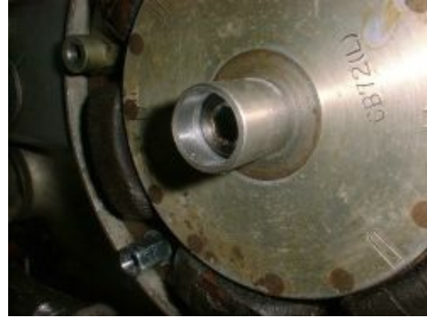
Figure 2 Mounting the driver sleeve.
