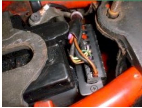
Figure 2 Ignition box mounting suggestion.
