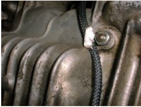
Figure 2.j Pickup lead protection.
