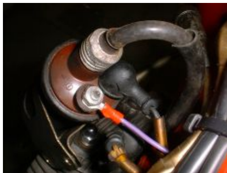
Figure 3 Mounting suggestion of the left ignition coil.
