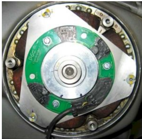
Figure 2.d Mounting the pickup (image shows older version, current version looks slightly different).
