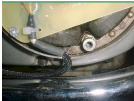
Figure 2.g Routing the pickup lead through the cutout.
