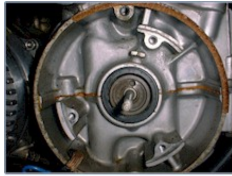
Figure 2.b Removal of the original sleeve so that our driver sleeve can be mounted.
