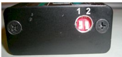
Figure 4 DIP switches and advance curve selection.
