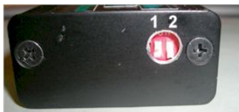
Figure 4 DIP switches and advance curve selection.
