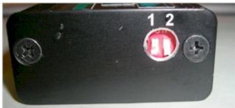
Figure 4 DIP switches and advance curve selection.
