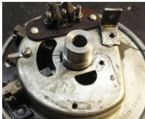
Push the sleeve onto the generator rotor and fasten it with the centre screw.
