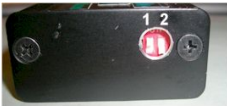
Figure 4 DIP switches and advance curve selection.
