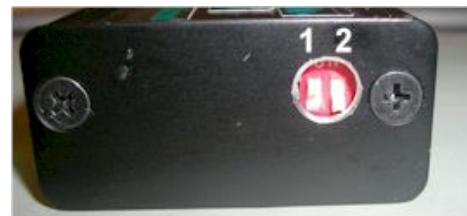
Figure 4 DIP switches and advance curve selection.
