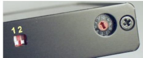
Figure 4 DIP switches and rotary switch.
